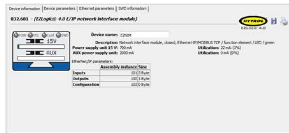
Figure 10: Select a proper device name to match on the PLC's configuration.
